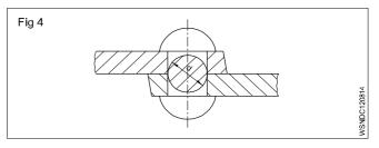
Rivet cross-section is the hole cross-section.
