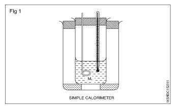
The apparatus used to measure the amount of heat by mixer method is called calorimeter. It is nothing but cylindrical shaped vessel and a stirrer made out of mostly copper.
