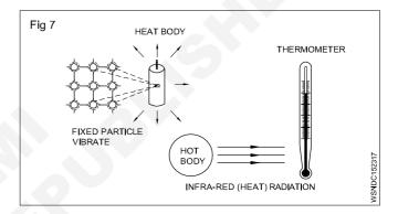
Transmission of heat takes place in three ways Conduction, Convection and Radiation.
